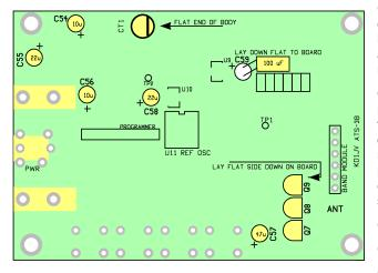
**C59:** 100 ufd aluminum electrolytic. Standing this cap up will cover the leads of U9, making them difficult to access if need be at some time. Therefore, mount the cap on it's side, angeling the leads slightly so the body of the cap is above the row of chip parts along it. Long lead is +
